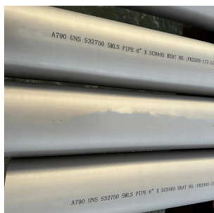
ASTM A790 UNS S32750 seamless pipe with heat-number marking
