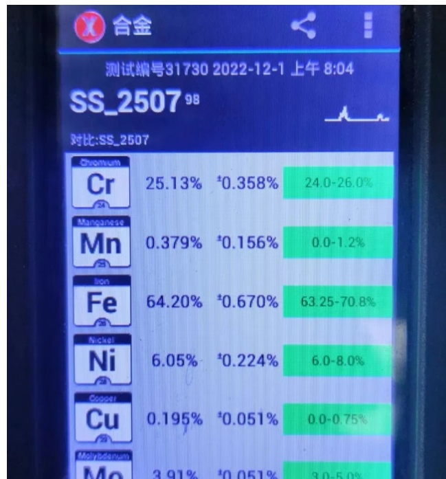
Portable XRF analyzer confirming UNS S32750 (SS_2507) chemistry on production stock
